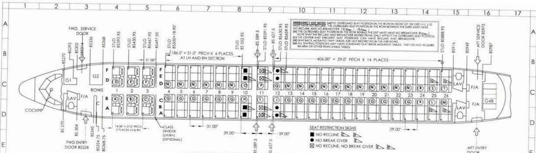
8737-401/PAXS CABIN CONFIGURATION FOR 150 PAXS ( 12 BUSINESS + 138 TOURIST ) SEATS, GALLEYS AND FURNITURES DISTRIBUTION - VIEW LOOKING DOWN
